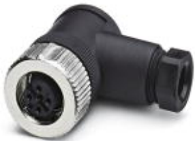
Sensor/actuator connector female, angled, 4-pos., M12-SPEEDCON, A-coded, screw connection, metal knurl, cable screw connection Pg7
