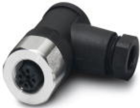
Sensor/actuator connector, female, angled, 4-pos., M12, screw connection, high-grade steel knurl, cable screw connection Pg7
