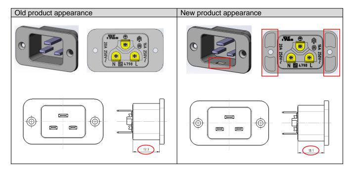
As the V-Lock notch and material for enhanced glow wire tests will be standard features, the material numbers with index .15 and .21 are obsolete and will be replaced by the standard numbers:
