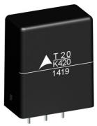
The T20 components are suitable for voltages between 130  $V_{RMS}$ and 1000 V<sub>RMS</sub>. Their surge current capability is up to 10,000 A (8/20 µs) and their power dissipation is 1.0 W. Depending on the voltage, the dimensions range from 22 mm x 26 mm x 12 mm to 27.5 mm x 27.5 mm x 18.5 mm.
