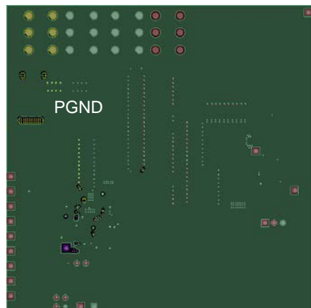
Figure 49f: IRDC3847 Demo board Layout Considerations – Mid Layer 4
