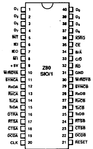
Figure 4. 40-pin Dual-In-Line Package (DIP), Pin Assignments
