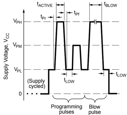
Figure 4. Programming pulse definition (see table 1)
