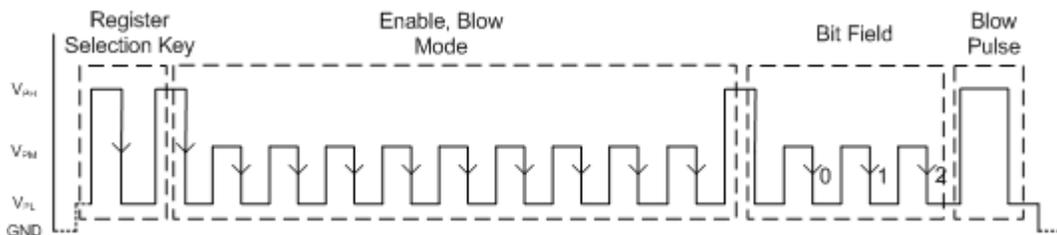
Figure 12. Example of Blow mode pulse sequence, Register Key = B<sub>OP</sub> selection bit field 2 (code 4)
