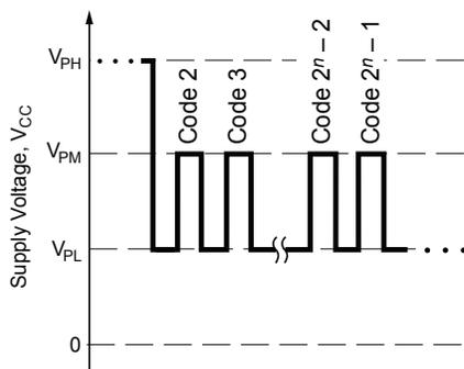
Figure 6. Try mode bit field addressing pulses
