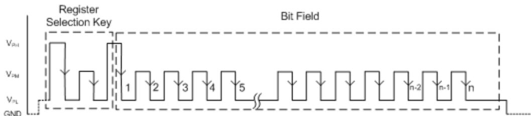
Figure 11. Example of Try mode pulse sequence, Register Key = B<sub>OP</sub> selection down counting
