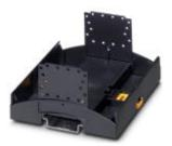
Installation component housing with vents, Lower part, Cross connection: DIN rail bus connector, Color: black, Width: 53.6 mm, Constructional height: 49 mm, Number of positions cross connector: 16
