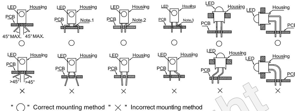
Note 1-3: Do not route PCB trace in the contact area between the leadframe and the PCB to prevent short-circuits.
