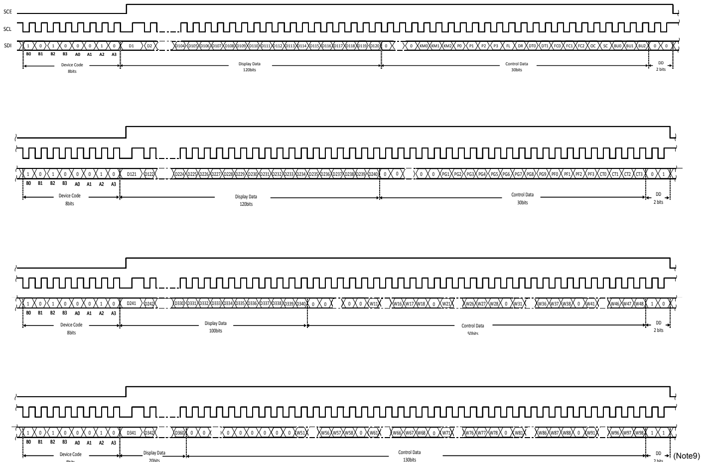
Figure 10. 3-SPI Data Transfer Format
