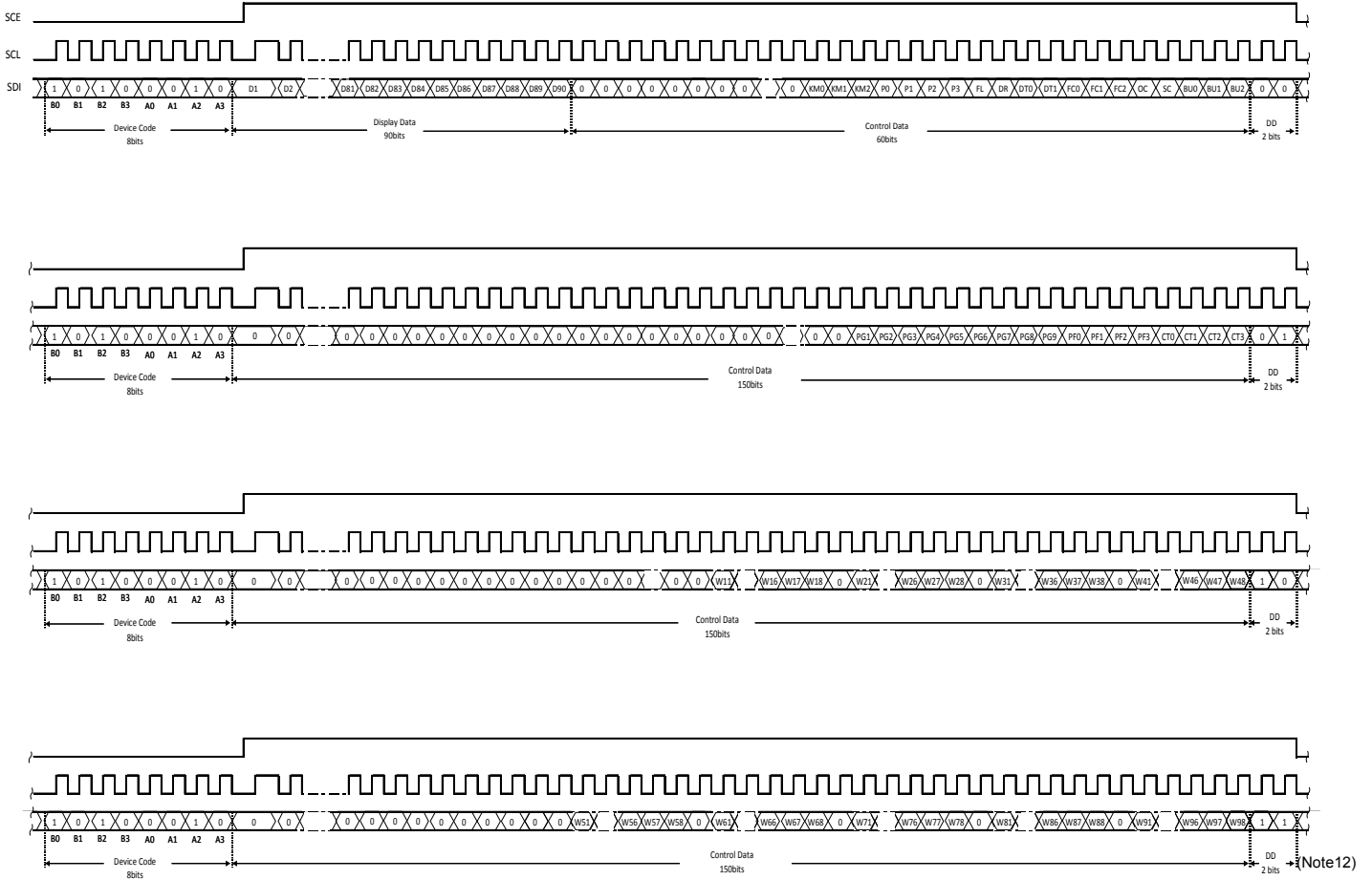
Figure 13. 3-SPI Data Transfer Format
