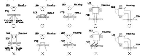
" $\bigcirc$ " Correct mounting method "imes" Incorrect mounting method
