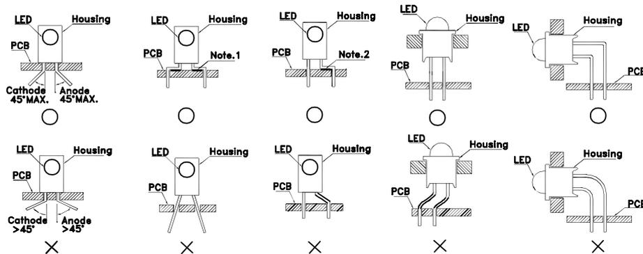
”O” Correct mounting method ”X” Incorrect mounting method
