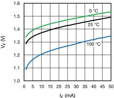
Fig. 7 - LED Forward Voltage vs. LED Forward Current
