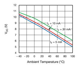
Fig. 4 - Output Open Circuit Voltage vs. Ambient Temperature
