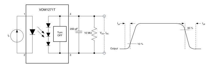
Fig. 1 -  $t_{\text{on}},\,t_{\text{off}}\,\text{Test}$  Circuit and Waveforms
