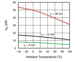
Fig. 3 - Output Short-Circuit Current vs. Ambient Temperature
