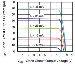
Fig. 8 - Short Circuit Output Current vs. Open Circuit Output Voltage
