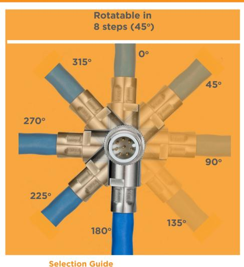
**Temperature Range** -40°C to 70°C **Current rating:** D-4: 4A / A-8: 2 A **Operational Voltage:** A-5 / D-4: 50 V DC / A-8: 30 V DC **Contact Resistance:** ≤ 5 mΩ Insulation resistance: >100 mΩ Data transmission characteristics: Class D according to IEC 11801:2002 Data transmission rate: 10/100 Mbit/s IP rating: IP67 Mating Cycles:  $\geq$  100 mating cycles **Standards:** EN 61373 Class 1
