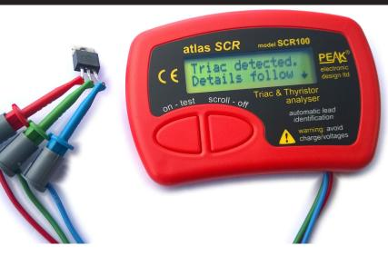
Thyristors and triacs vary a great deal in their requirements for gate trigger currents, some can be triggered with just  $50\mu A$ , others may need higher test currents. This instrument can generate gate test currents up to 90mA. The latching and holding test current is nominally 100mA.
