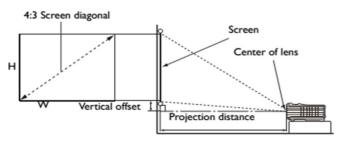
The screen aspect ratio is 4:3 and the projected picture is in a 4:3 aspect ratio
