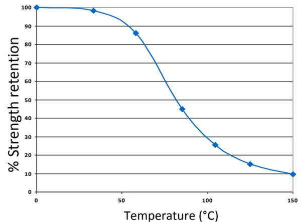
ET514 can withstand higher temperatures for brief periods (such as for paint baking and wave soldering processes) providing the joint is not unduly stressed. The minimum temperature the cured adhesive can be exposed to is -40°C (-40°F) depending on the materials being bonded.
