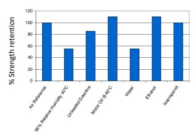
Specimens were immersed for 1000 hours at 22°C (unless otherwise stated).
