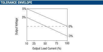
The voltage tolerance envelope shows typical load regulation characteristics for this product series. The tolerance envelope is the maximum output voltage variation due to changes in output loading.
