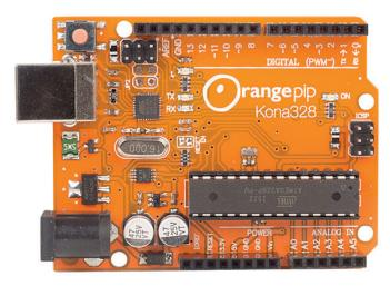
**LED: 13** There is a built-in LED connected to digital pin 13. When the pin is HIGH value, the LED is on, when the pin is LOW, it's off.
