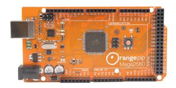
External Interrupts: 2 (interrupt 0), 3 (interrupt 1), 18 (interrupt 5), 19 (interrupt 4), 20 (interrupt 3), and 21 (interrupt 2) These pins can be configured to trigger an interrupt on a low value, a rising or falling edge, or a change in value. See the attachInterrupt() function for details.
