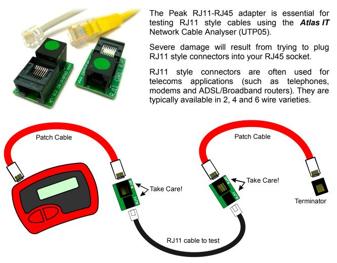
It is common for RJ11 terminated cables to be wired in a mirrored format although straightthrough connections are also in use.
