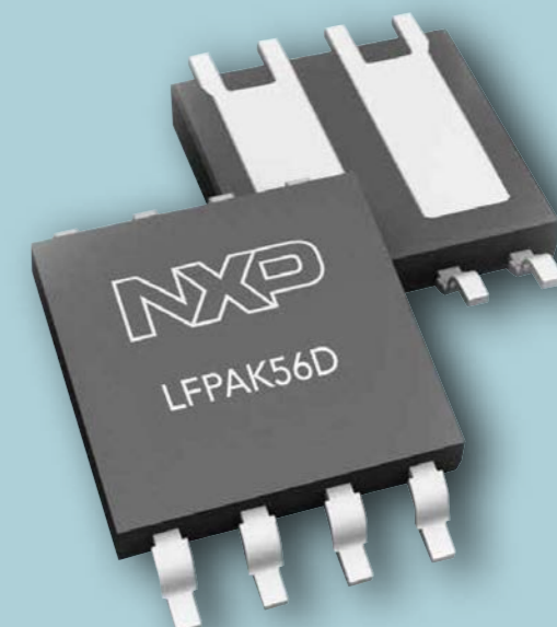
LFPAK56D (SOT1205) Dual package 5 x 6 x 1.1 mm
