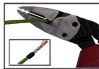
Crimping of ferrules 1.5 + 2.5mm 2
