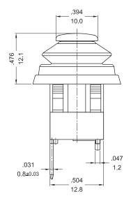
Dimensions : Inches/Millimetres Tolerances ±0.012"/0.3mm
