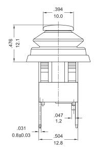
Dimensions : Inches/Millimetres Tolerances ±0.012"/0.3mm
