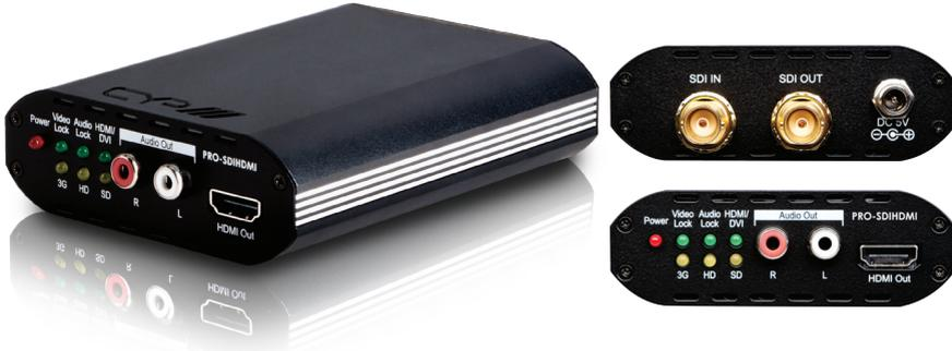
The PRO-SDIHDMI Converter accepts SD-SDI, HD-SDI, and 3G-SDI signals and converts to HDMI. The SDI input also has a bypass which is outputted simultaneously alongside the HDMI output allowing the SDI signal to be extended over distances up to 300m. This device also has the added benefit of an integrated audio de-embedder for sending 2-channel (L/R) audio to an AV amplifier.
