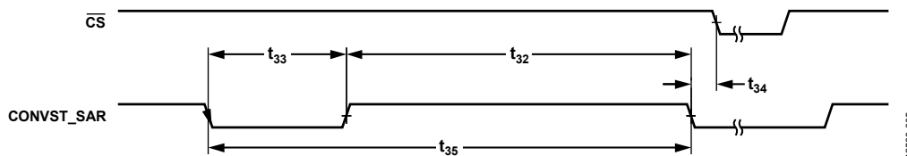
Figure 5. SAR ADC Timing Diagram
