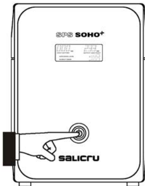
Fig. 11. Start up and shutdown.
