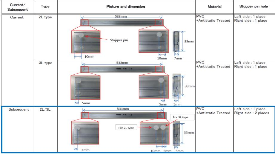
Dimension and material is same. Subsequent 2L/3L type has two stopper pin hole at right side.
