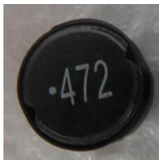
Marking with Pad-Printing
