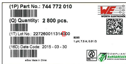
Label example for pad printing (13 th digit marked in red)
