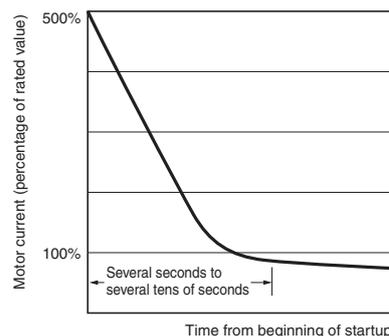
For a motor with a rating of 5 A, the startup current will be approximately 30 A. The startup current will exceed the overload capacity (rating: 150% for 1 s) of the K8DT-AW1 and K8DT-AW2 and result in failure of the Relay. To monitor the motor load, use the K8DT-AW3. (Overload capacity: 120% of rating for continuous load, 200% of rating for 30 s, and 600% of rating for 1 s). The K8DT-AW3 has a large input range. Pass the conductors multiple times through the special CT.
