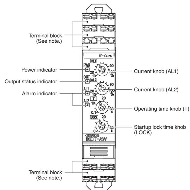
**Note:** Use solid wires, stranded wires, or ferrules to connect to the terminals.
