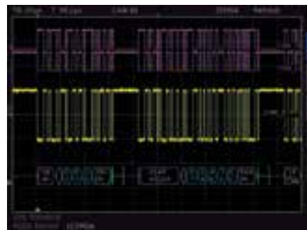
HEX decoded CAN bus signal.
