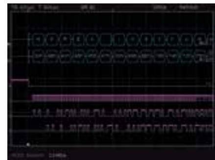
SPI bus signal, MISO / MOSI decoded.
