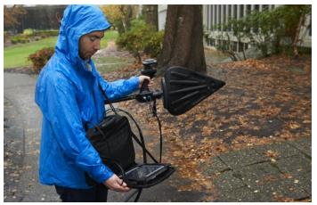
Combined with a Tektronix USB spectrum analyzer, the Alaris DF-A0047 direction finding antenna makes interference hunting easy. Lines of bearing are automatically transmitted from the antenna to SignalVu-PC Map software, enabling fast triangulation on interference sources.
