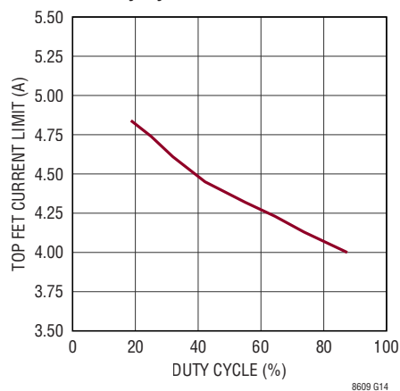
Top FET Current Limit vs Duty Cycle
