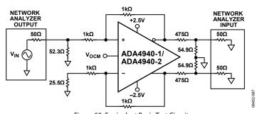
Figure 59. Equivalent Basic Test Circuit
