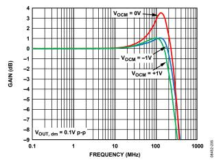
Figure 15. Small Signal Frequency Response for Various V<sub>OCM</sub> (SOIC)
