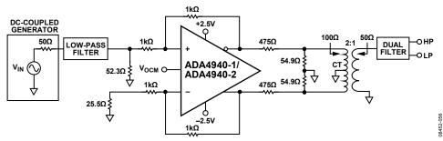
Figure 60. Test Circuit for Distortion Measurements
