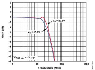
Figure 24. V<sub>OCM</sub> Large Signal Frequency Response for Various Supplies
