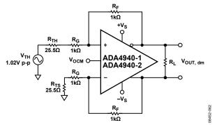
Figure 69. Thevenin Equivalent and Matched Gain Resistors
