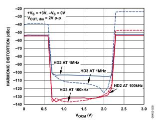
Figure 35. Harmonic Distortion vs.  $V_{\text{OCM}}$  for 100 kHz and 1 MHz, 3 V Supply (LFCSP)
