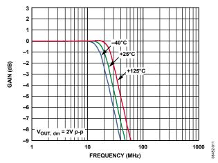
Figure 12. Large Signal Frequency Response for Various Temperatures
