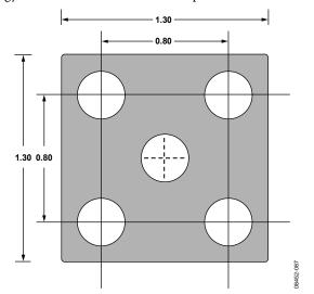
Figure 75. Recommended PCB Thermal Attach Pad Dimensions (mm)
