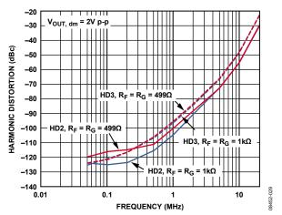
Figure 36. Harmonic Distortion vs. Frequency for Various R<sub>F</sub> and R<sub>G</sub> (LFCSP)
