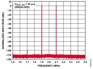
Figure 37. 2 MHz Intermodulation Distortion (LFCSP)
