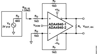
Figure 66. Calculating Single-Ended Input Impedance, R<sub>IN</sub>
