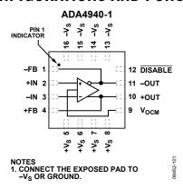
Figure 4. ADA4940-1 Pin Configuration (16-Lead LFCSP)
