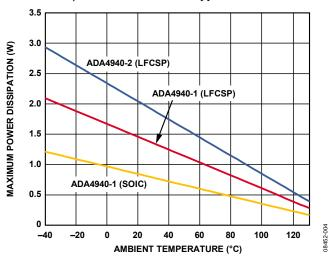
Figure 3. Maximum Safe Power Dissipation vs. Ambient Temperature
