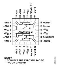
Figure 6. ADA4940-2 Pin Configuration (24-Lead LFCSP)
