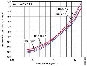
Figure 28. Harmonic Distortion vs. Frequency vs. Gain (SOIC)
