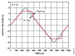
Figure 43. Output Overdrive Recovery, G = 2
