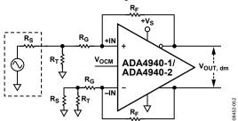
Figure 65. ADA4940-1/ADA4940-2 Configured for Unbalanced (Single-Ended) Input
