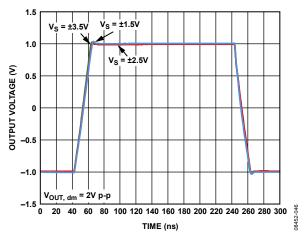
Figure 53. Large Signal Transient Response for Various Supplies
