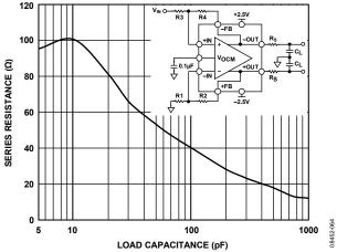
Figure 71. Capacitive Load vs. Series Resistance (LFCSP)
