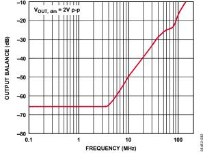
Figure 39. Output Balance vs. Frequency
