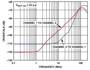
Figure 40. Crosstalk vs. Frequency, ADA4940-2
