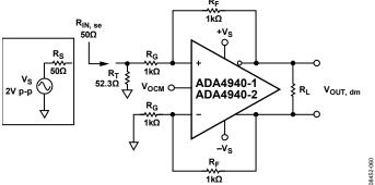
Figure 67. Adding Termination Resistor R<sub>T</sub>
