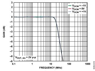
Figure 17. Large Signal Frequency Response at Various  $V_{\text{OCM}}$  Levels
