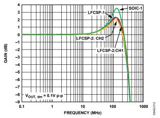
Figure 13. Small Signal Frequency Response for Various Packages
