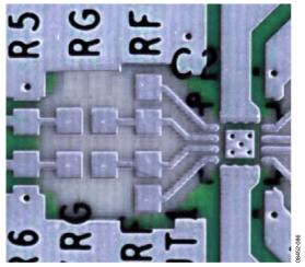
Figure 74. Ground and Power Plane Voiding in Vicinity of R<sub>F</sub> and R<sub>G</sub>
