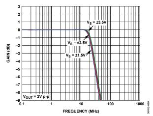
Figure 11. Large Signal Frequency Response for Various Supplies
