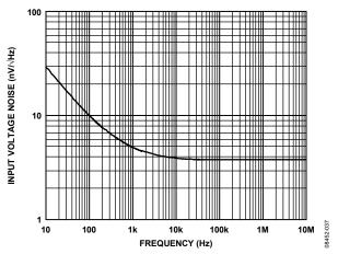
Figure 44. Voltage Noise Spectral Density, Referred to Input
