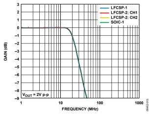
Figure 16. Large Signal Frequency Response for Various Packages
