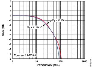
Figure 21. V<sub>OCM</sub> Small Signal Frequency Response for Various Supplies
