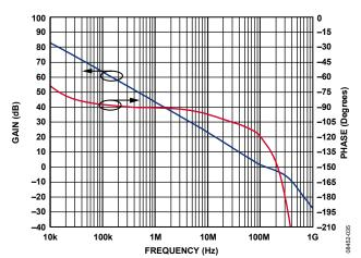
Figure 42. Open-Loop Gain and Phase vs. Frequency
