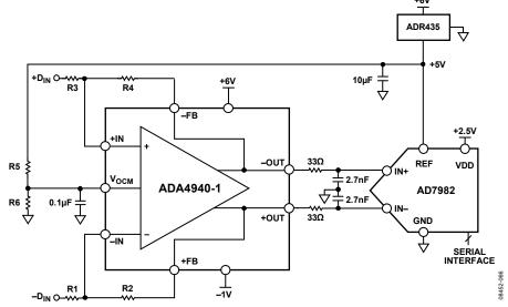
Figure 73. ADA4940-1 (LFCSP) Driving the AD7982 ADC
