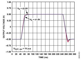
Figure 58. V<sub>OCM</sub> Large Signal Transient Response
