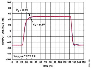
Figure 56. V<sub>OCM</sub> Small Signal Transient Response
