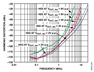
Figure 33. Harmonic Distortion vs. Frequency for Various V<sub>OUT, dm</sub> (LFCSP)
