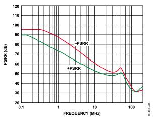
Figure 41. PSRR vs. Frequency
