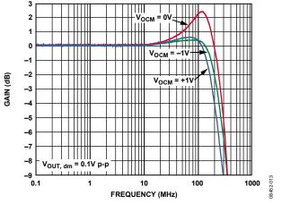
Figure 14. Small Signal Frequency Response at Various V<sub>OCM</sub> Levels (LFCSP)
