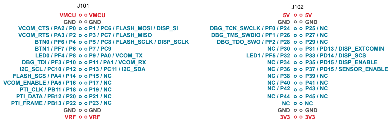
Figure 4.2. Radio Board Pin Mapping on Breakout Pads
