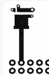
Figure 5. Minimum Pads of 2-ounce Copper
