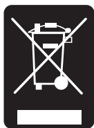
Fig. 1.4: Product labeling in accordance with EN 50419
