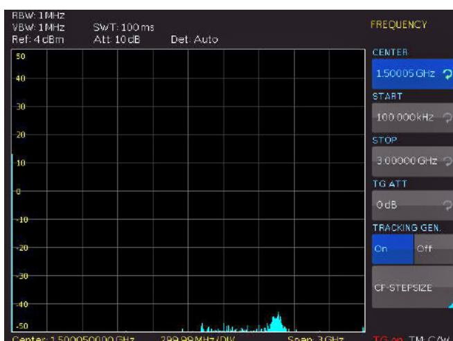
Fig. 6.11: Loosening of the RF cable completely
