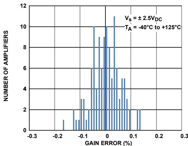
FIGURE 7. PGIA GAIN ERROR DISTRIBUTION,  $G = 100$
