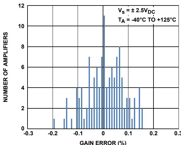
FIGURE 5. PGIA GAIN ERROR DISTRIBUTION,  $G = 1$
