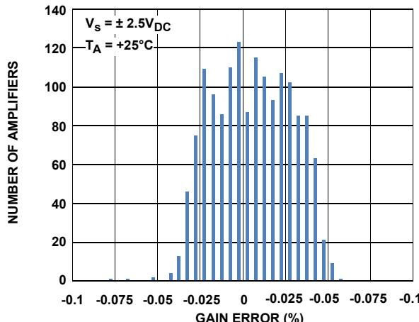
FIGURE 9. PGIA GAIN ERROR DISTRIBUTION,  $G = 1 \text{ TO } 1,000$
