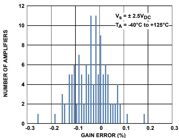
FIGURE 8. PGIA GAIN ERROR DISTRIBUTION,  $G = 1,000$
