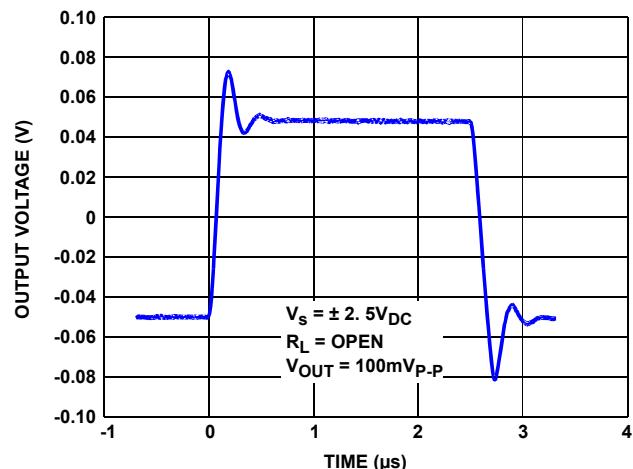
FIGURE 65. OP AMP SMALL SIGNAL TRANSIENT RESPONSE
