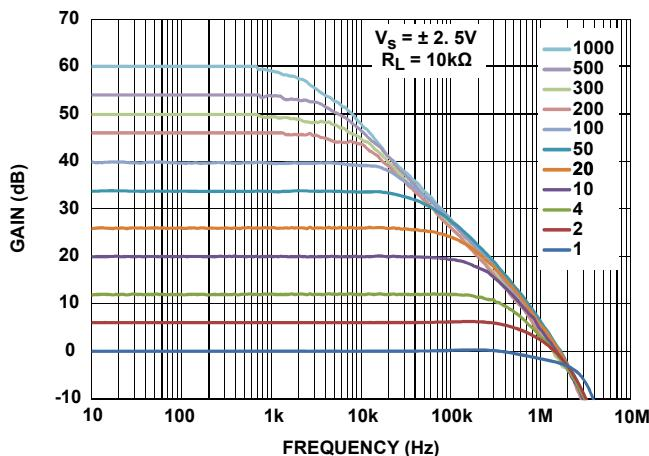
FIGURE 35. PGIA GAIN VS FREQUENCY vs GAIN SETTINGS
