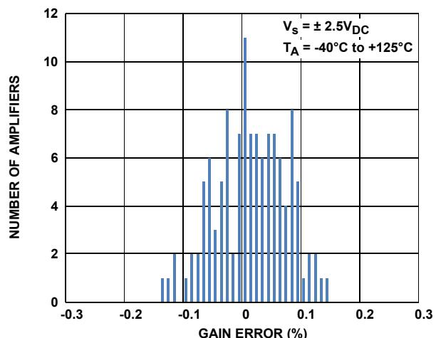
FIGURE 6. PGIA GAIN ERROR DISTRIBUTION,  $G = 10$
