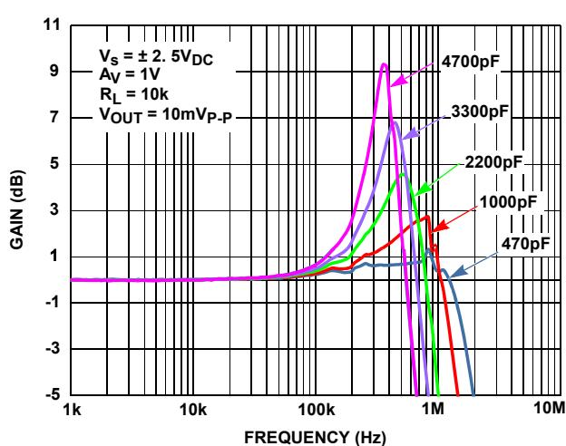
FIGURE 40. PGIA GAIN vs FREQUENCY vs CL, ISL2863x
