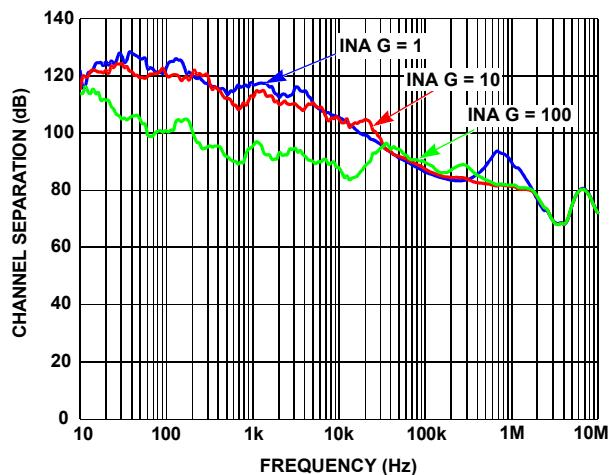
FIGURE 54. CHANNEL SEPARATION vs FREQUENCY, HOSTILE
