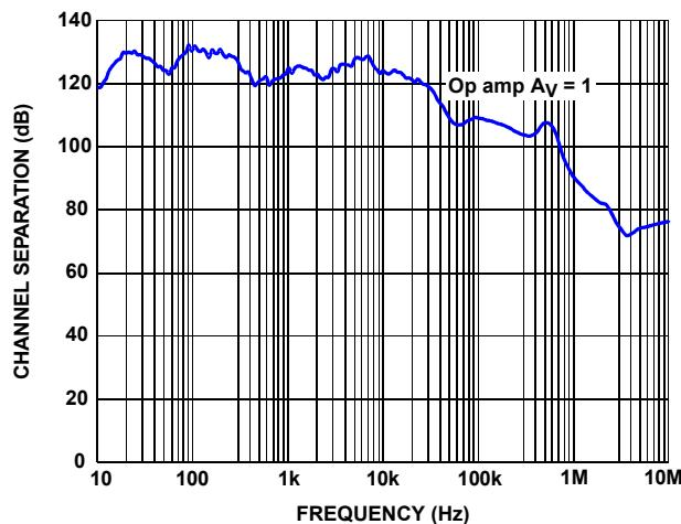
FIGURE 53. CHANNEL SEPARATION vs FREQUENCY, HOSTILE INA,
