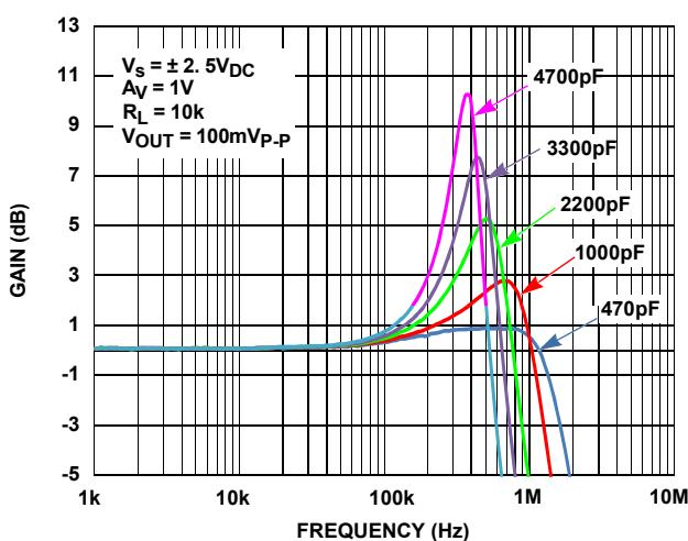
FIGURE 39. PGIA GAIN vs FREQUENCY vs CL, ISL2853x
