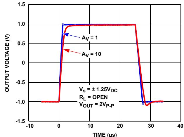
FIGURE 66. OP AMP LARGE SIGNAL TRANSIENT RESPONSE
