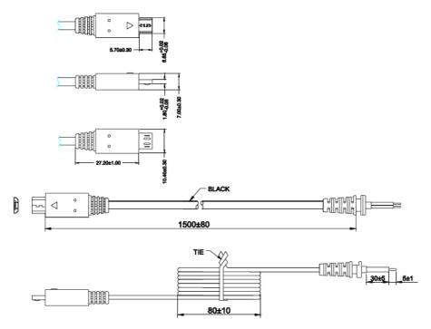
NOTE:1.WIRE TYPE:VW-1 80°C 300V L=1500mm 1185 3.5Ø 18AWG BLACK 2.THE POLARITY:
