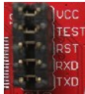
Figure 36. eZ430 Debug Connector on MSP-EXP430G2 LaunchPad
