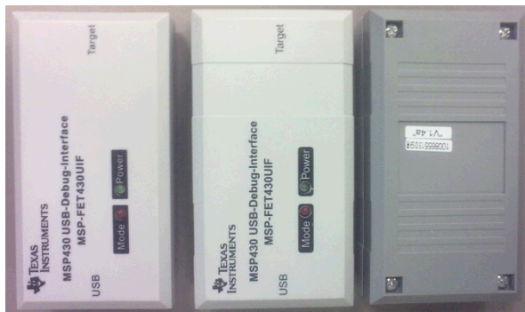
Figure 20. MSP-FET430UIF Version 1.4a Top and Bottom Views
