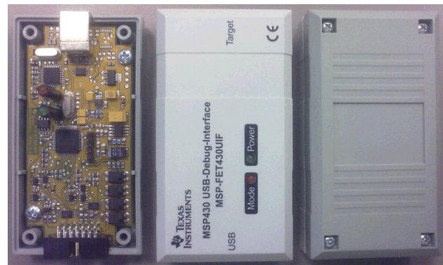
Figure 21. MSP-FET430UIF Version 1.3 Top and Bottom Views
