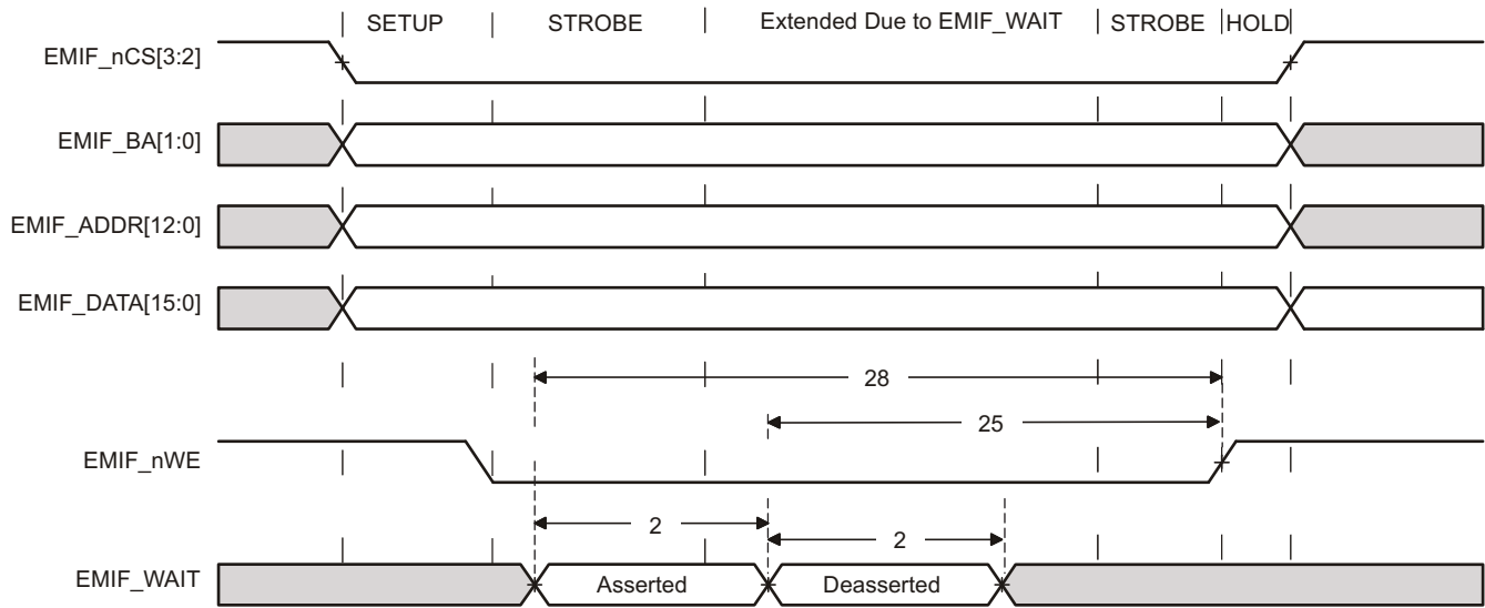
Figure 6-16. EMIFnWAIT Write Timing Requirements
