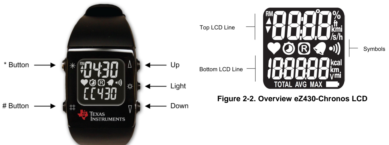
Figure 2-1. eZ430-Chronos Wrist Module Push Buttons
