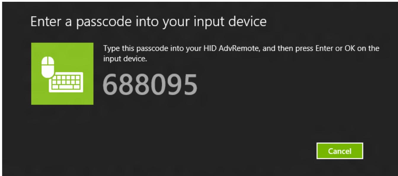
The advanced remote is paired with Windows and bond data is stored on both devices, making reconnecting faster and passcode entry unnecessary.
