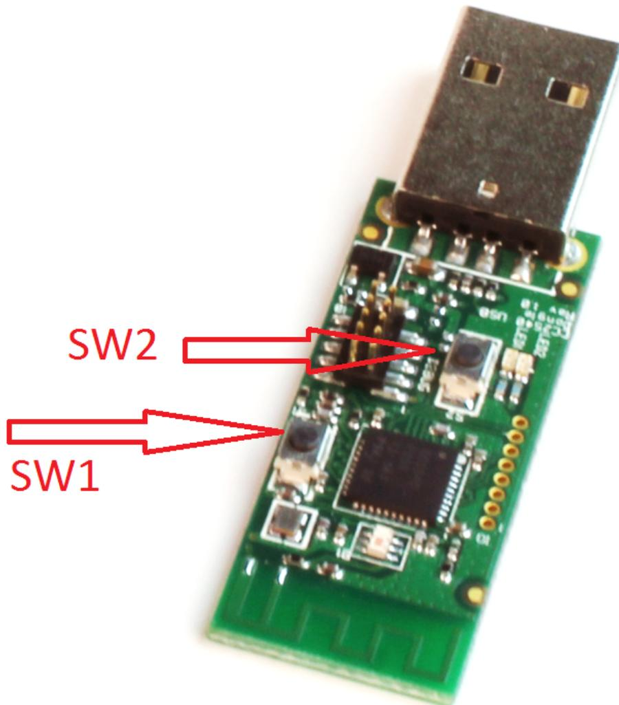
Pressing **SW2** on the dongle disconnects any active connection between the dongle and an advanced remote.
