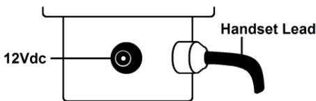
For power, the VM25UR has a 12Vdc input near to the hard-wired microphone lead. A DC lead is provided for powering from a vehicle cigar lighter socket and this should also be fed into the vehicle cabin through a window or bulkhead and connected to the 12Vdc outlet.
