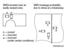
When placing a component near an area which is apt to bend or a grid groove on the PC board, it is advisable to have both electrodes subjected to uniform stress, or to position the component's electrodes at right angles to the grid groove or bending line (see c) Component orientation).
