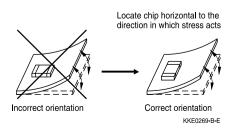
Choose a mounting position that minimizes the stress imposed on the chip during flexing or bending of the board.
