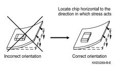
Choose a mounting position that minimizes the stress imposed on the chip during flexing or bending of the board.
