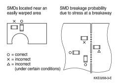
When placing a component near an area which is apt to bend or a grid groove on the PC board, it is advisable to have both electrodes subjected to uniform stress, or to position the component's electrodes at right angles to the grid groove or bending line (see c) Component orientation).
