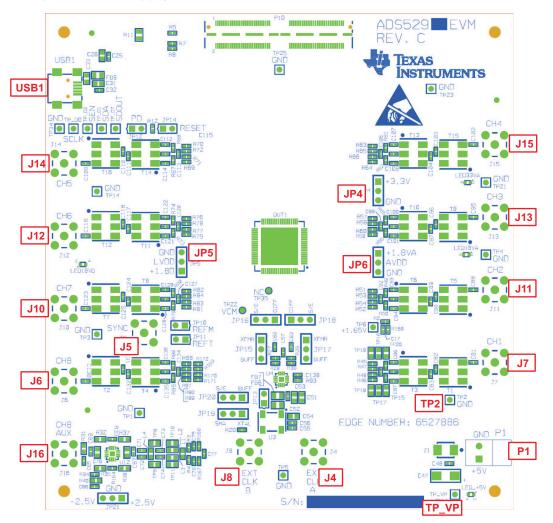
Figure 11. I/O, PWR, and USB Connector
