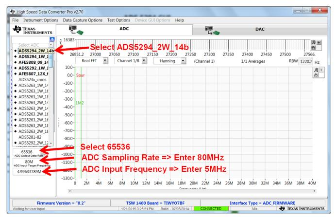
Figure 6. TSW1400 GUI Launch
