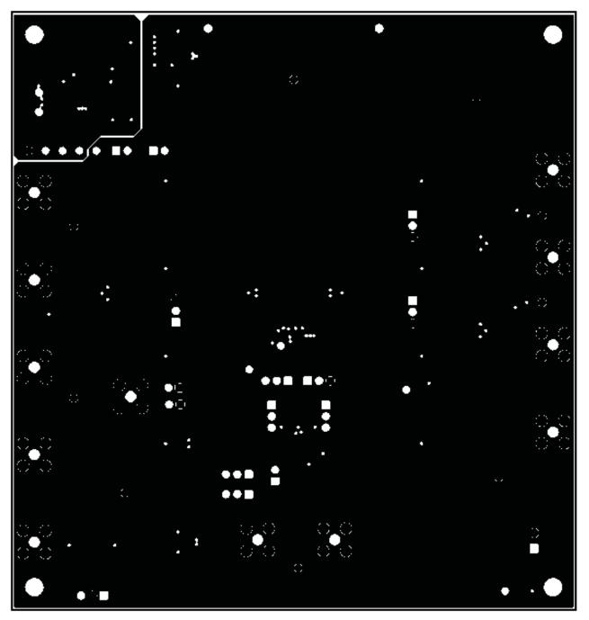
Figure 27. ADS5294EVM Internal Layer 1, Ground – Top View
