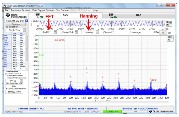
Figure 10. User Interface: Single FFT Format
