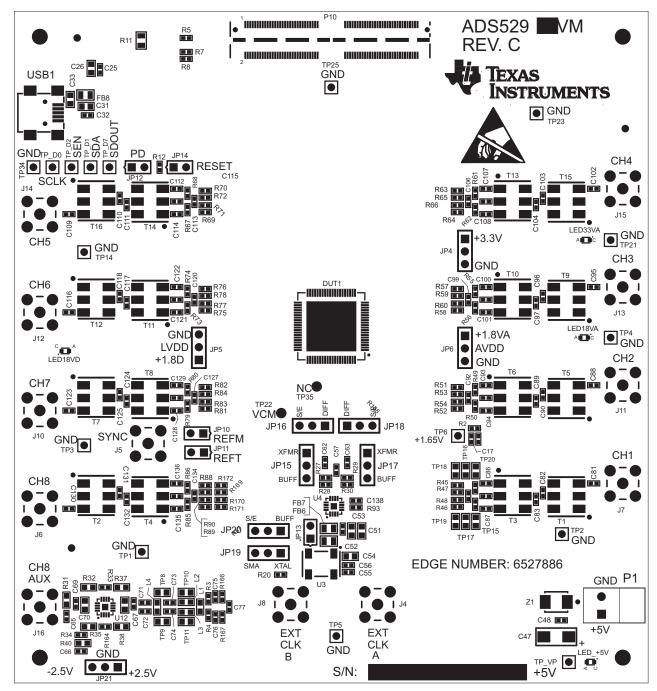
Figure 24. ADS5294EVM Top Layer Assembly Drawing – Top View
