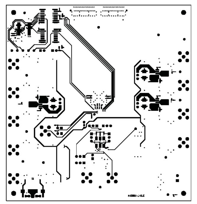
Figure 31. ADS5294EVM Bottom Layer Copper – Top View
