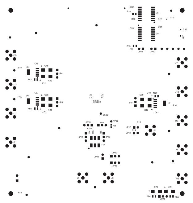
Figure 25. ADS5294EVM Bottom Layer Assembly Drawing – Bottom View
