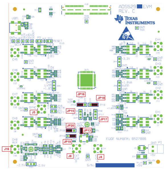
Figure 12. ADS5294EVM Default Clock Jumper Locations
