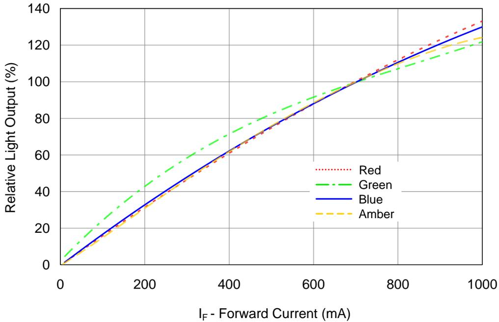
Figure 8: Typical relative light output vs. forward current @ T<sub>c</sub> = 25°C.
