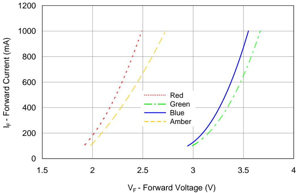
Figure 10: Typical forward current vs. forward voltage @ T<sub>c</sub> = 25°C.
