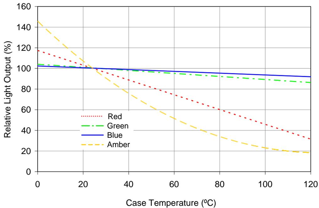
Figure 9: Typical relative light output vs. case temperature.
